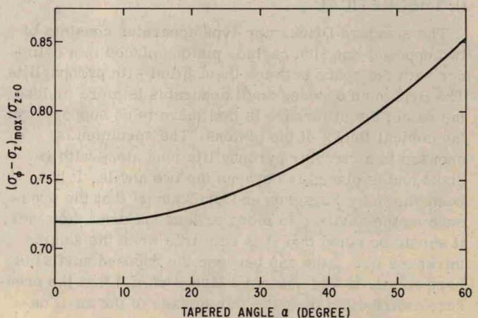
FIG. 2. The ratio of  $(\sigma_\theta - \sigma_z)_{\max}$  to  $\sigma_z$  at  $z=0$  as a function of tapered angle  $\alpha$ .
